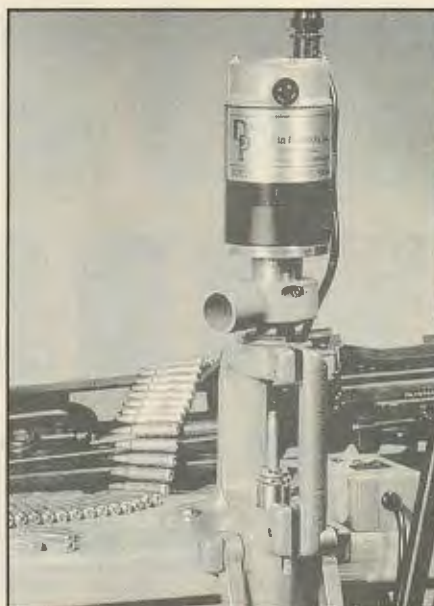
Brass cases must be trimmed. If the neck of a stretched case protrudes into the barrel's throat, it can lead to a potentially dangerous increase in chamber pressure. Dillon's Rapid Trim 1200B trims cases with the same stroke that resizes them.
